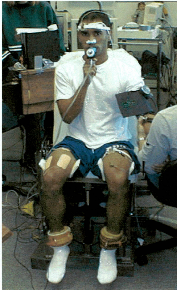
Figure 2. Subject utilizing the mouthpiece and nose clip of the Aerosport VO2000 portable metabolic cart to measure V_E , VO_2 , VCO_2 , and RQ during the 4-minute-long contractions.
